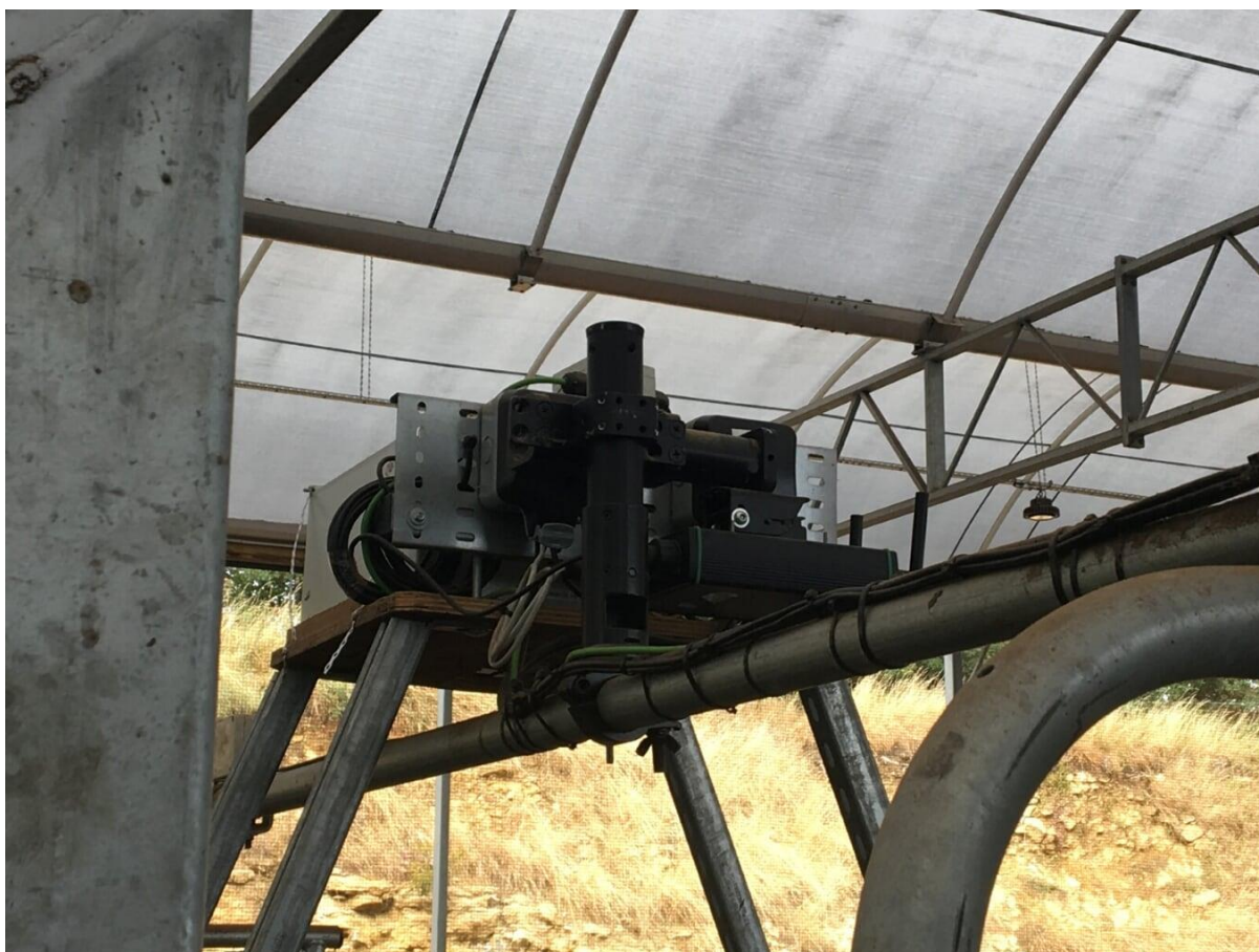
Fig 13. Body condition scoring camera positioned above automated cow sorting passage
