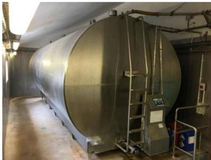
Bulk milk tank that had a sensor fit that milking could not commence without putting the pipe into the tank!
