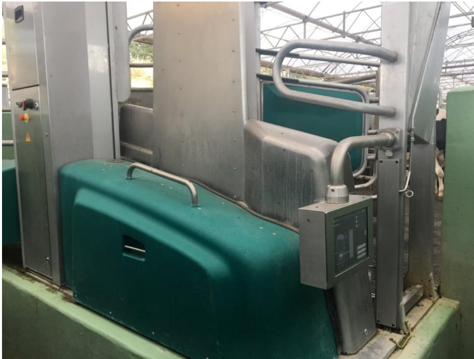
Fig 9. One of three milking robots with a touch screen to monitor milking and change settings
