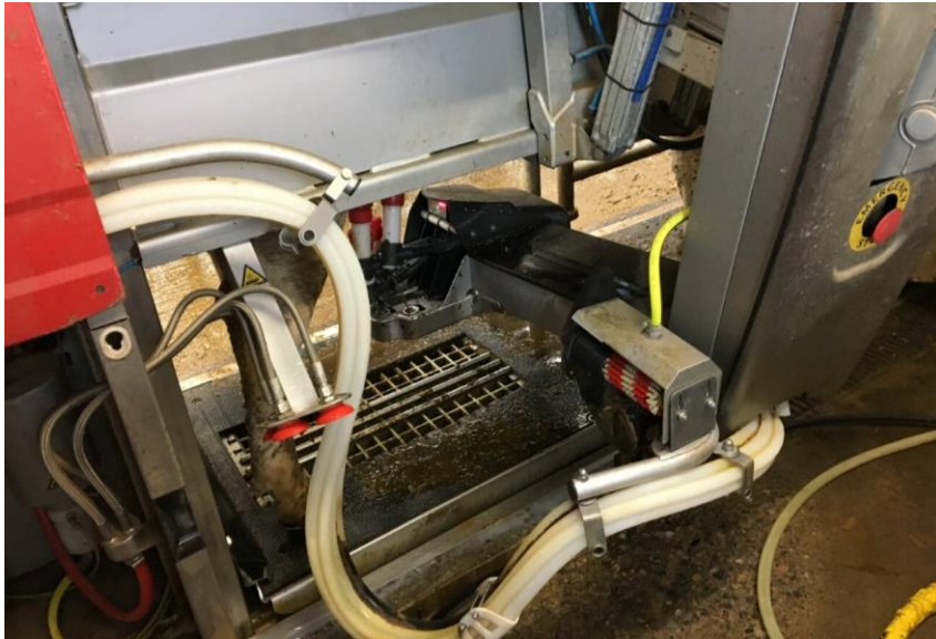
Fig 45. The Lely Astronaut Robotic Milker
