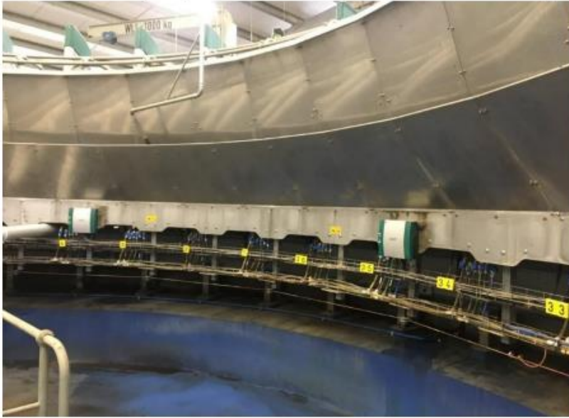
Inside of the rotary milking parlour accessible via an underpass
