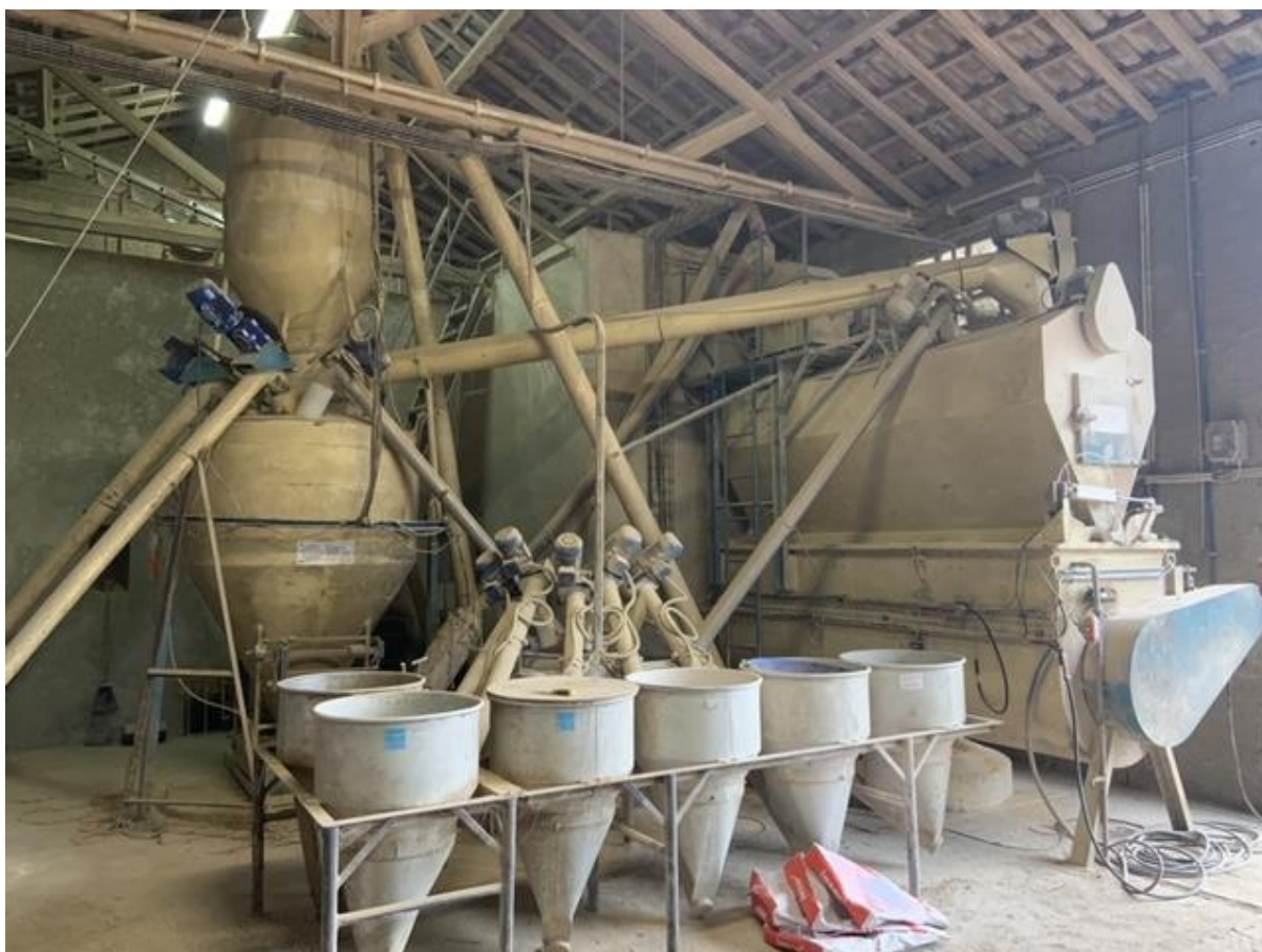
Figure 4. The specialist mill at Farm 1. The small hoppers are used to add small volume additives into the mix.
