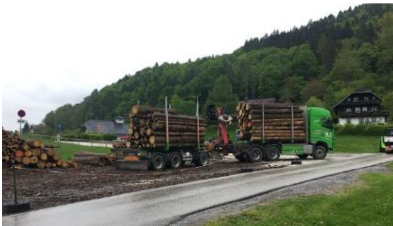
Lorry haulage from multiple cable crane extraction sites dropping timber in grading yard.
