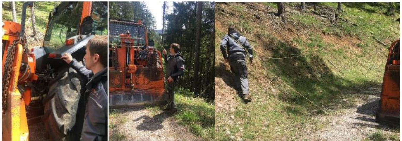
The auxiliary winch, fitted to a tractor-mounted timber winch, used for pulling the main winchline uphill.
