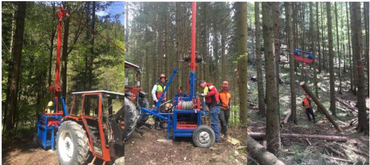
Small-scale self-built cable crane unit used for firewood extraction.
