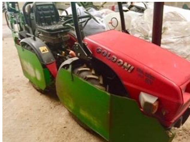
Goldoni forestry tractor with additional guards to prevent tree damage.
