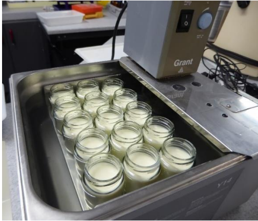
Fig 2. Glass jars filled with clotting milk, incubated in water bath at 32°C
