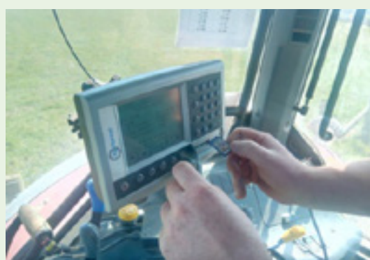
Field data was supplied to the lime spreading contractor through an SD card inserted into the tractor's GPS control panel.
