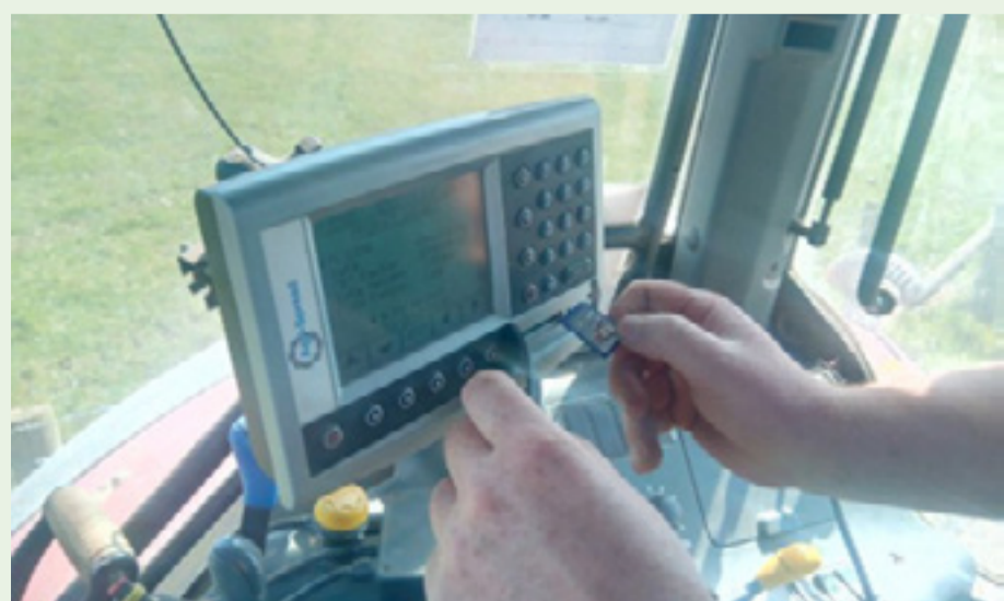
Figure 2: Transfer of soil mapping data to tractor GPS control panel on SD card.
