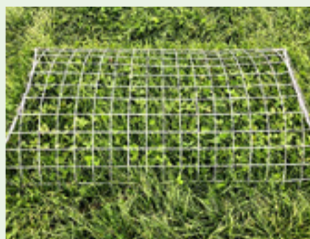
Figure 2. A cage in the white clover field used to exclude stock so growth rates can be measured.
