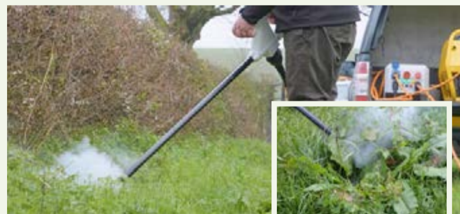
Figure 4. The RootWave Pro electrical weed er system was used in these trials, which sends a high voltage current through the plant effectively boiling all plant cells.
