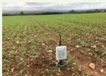
Figure 3: Set of soil nitrate, temperature and moisture sensors with LoRaWAN transmitter.
