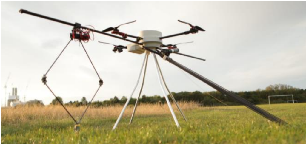
1 CropHopper combined UAV and flex legs source – haybeesee.com
