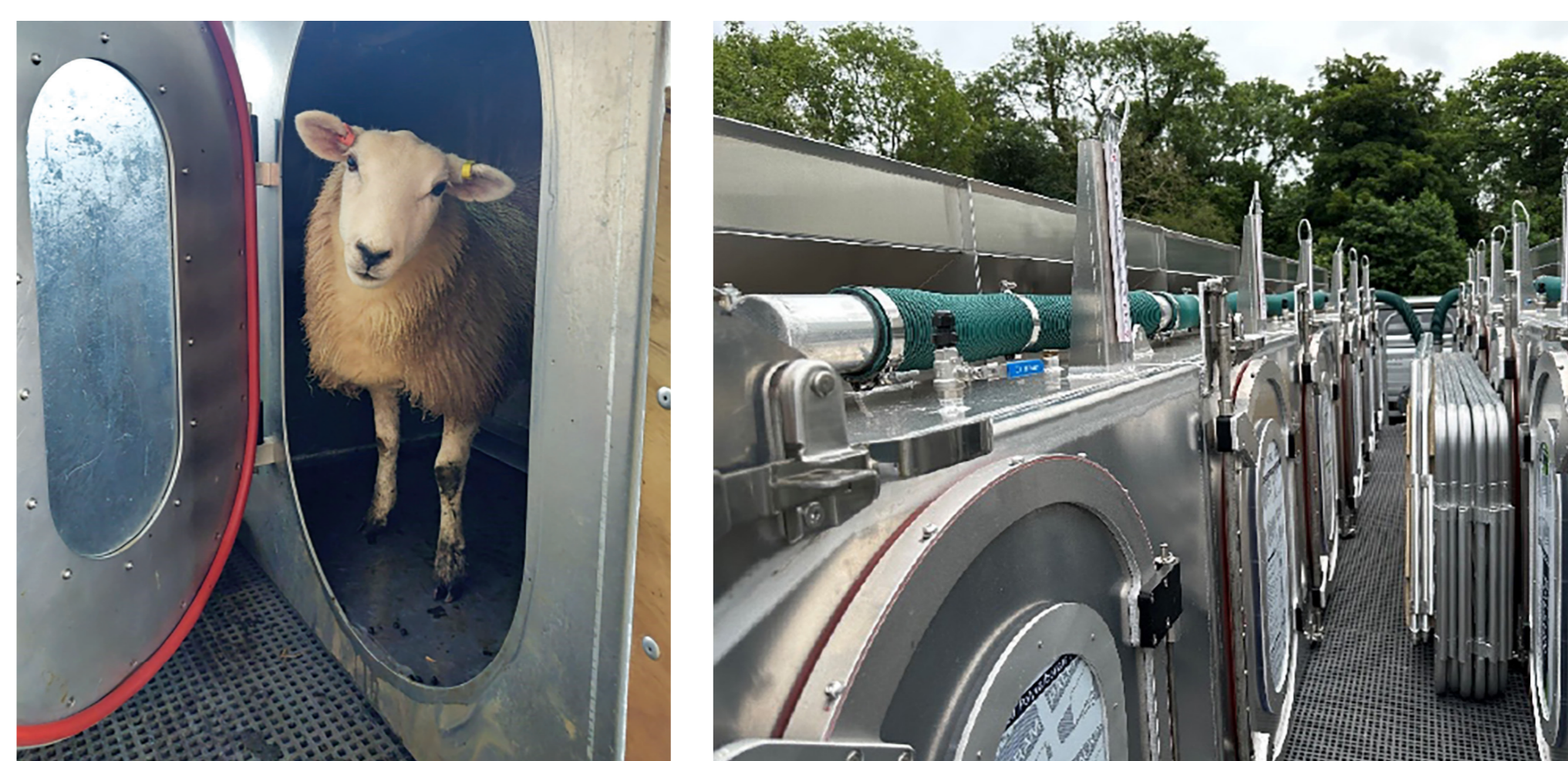
Portable Accumulation Chamber (PAC) is used to measure methane emissions in sheep
