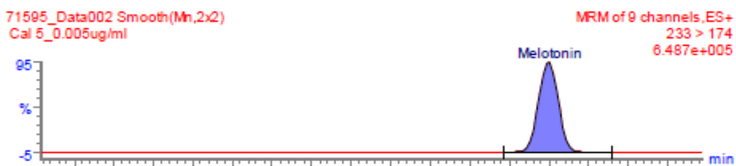
Figure 3. Example melatonin chromatography (233>174), in a solvent standard at 0.005 \mu\text{g/mL} .
