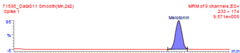
Figure 1. Example melatonin chromatography (233>174), in a fortified pasteurised milk sample at 0.01 \mu\text{g/mL} .
