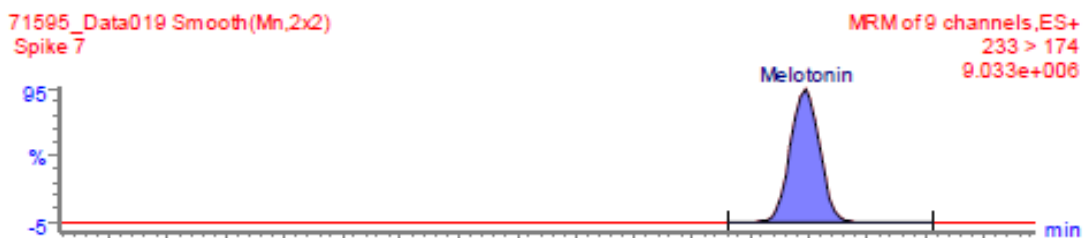
Figure 2. Example melatonin chromatography (233>174), in a fortified pasteurised milk sample at 0.1 \mu\text{g/mL} .
