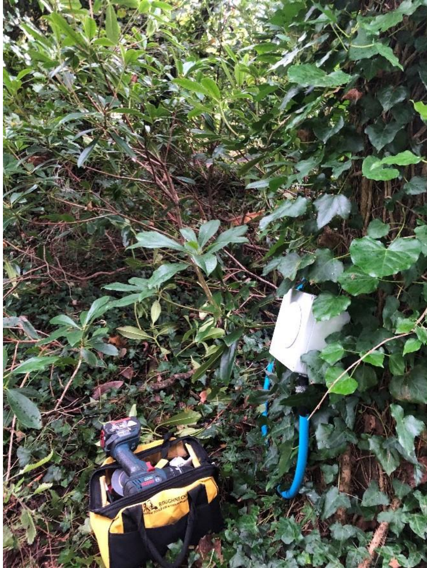
Prototype vehicle detector transmitter in hedgerow
