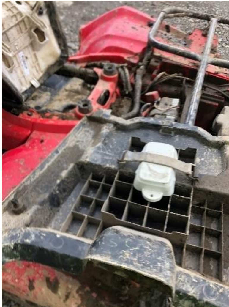
Digital Matter Oyster GPS Tracker mounted on quad bike
