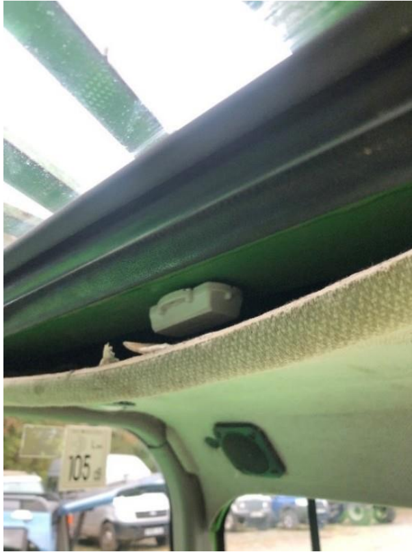
Digital Matter Guppy Movement Sensor in telehandler
