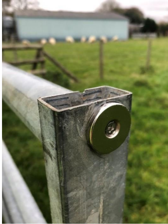
Gate open close sensor on gate
