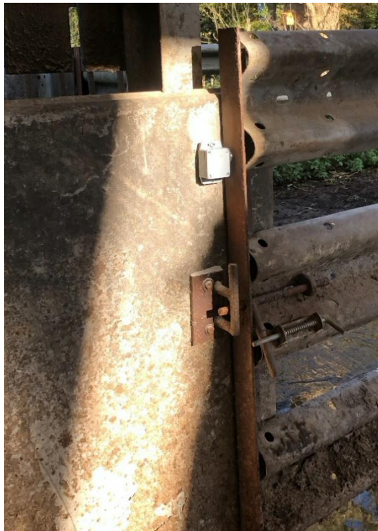
Open close sensor on gate post
