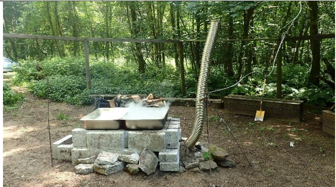
Wood stove in operation with two 45 litre Gastronorm pans
