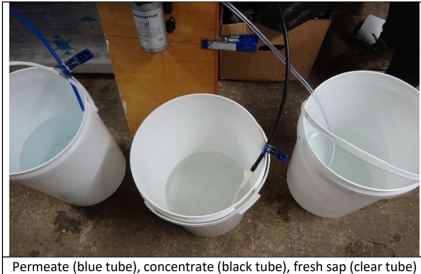
Figure 7: Separating sap into concentrate and permeate using RO
