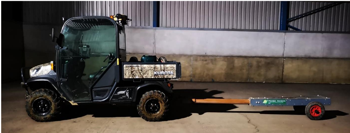
Figure 1: Kubota RTV vehicle with GPS auto steer guidance and EM Conductivity sensor.
