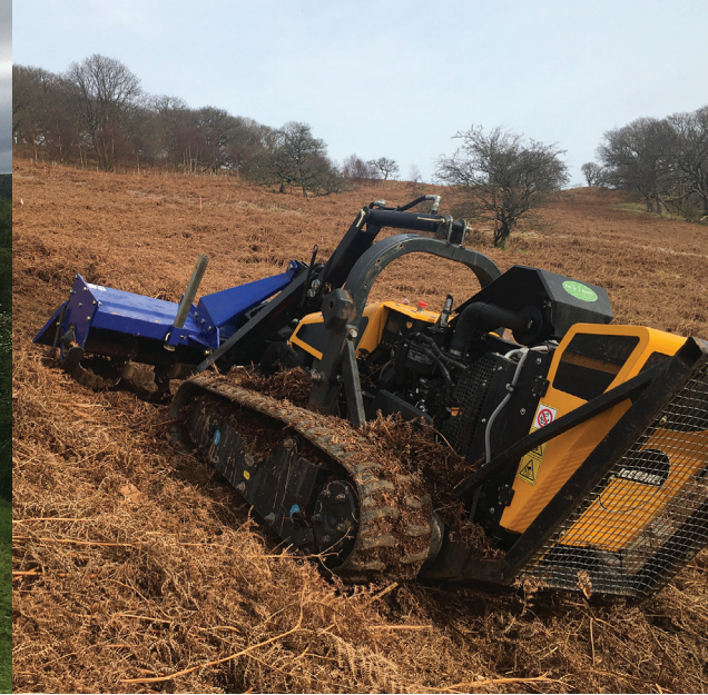
The remote controlled Robocut machine with a rotavator attachment.
