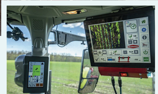
The vision guidance system of the Steketee weeder.
