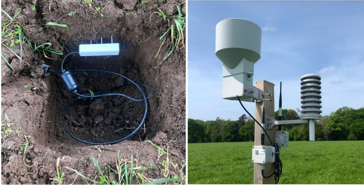
Figure 8: Image of the soil sensor (left) and air and rainfall sensors (right)
