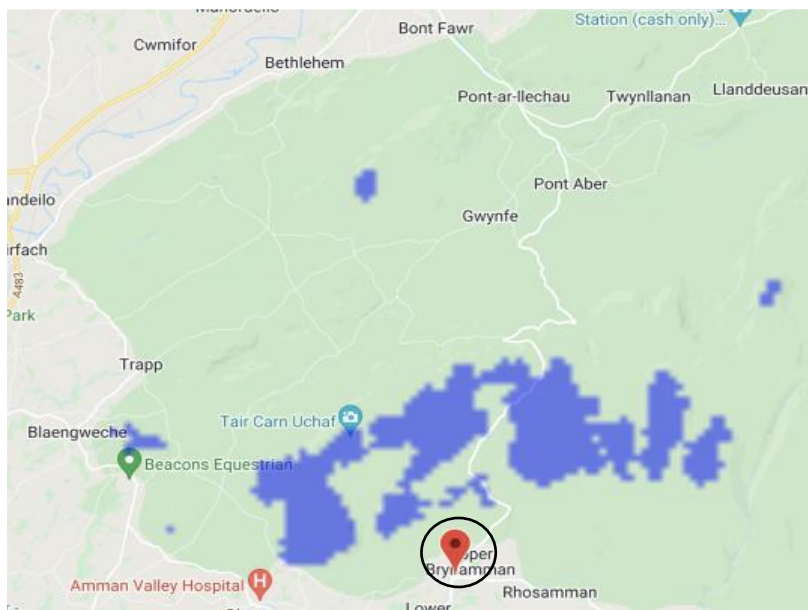
Figure 9: Sigfox coverage (blue) across an area of Wales including the Black Mountains. Antenna circled.
