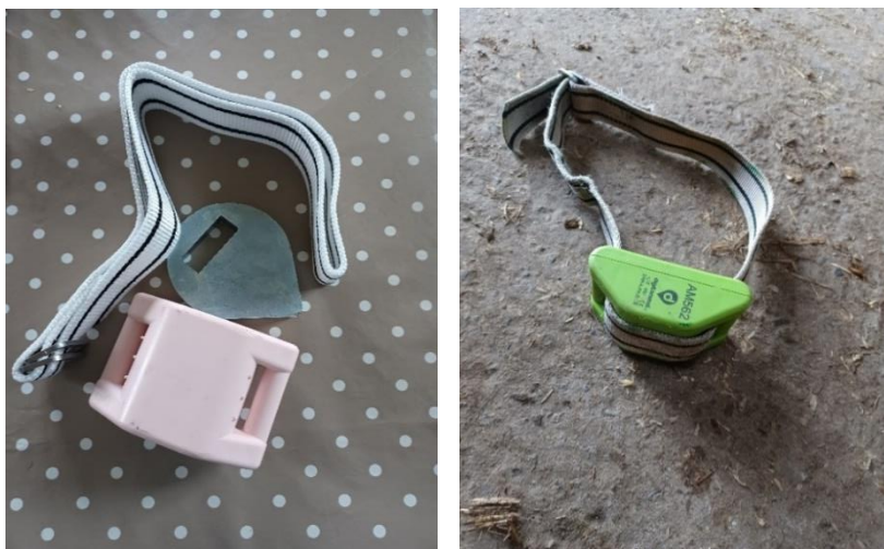
Figure 8: Digitanimal collars used on both cattle and sheep. The left photo also shows the weight available to attach to the collar to position the product better on sheep.
