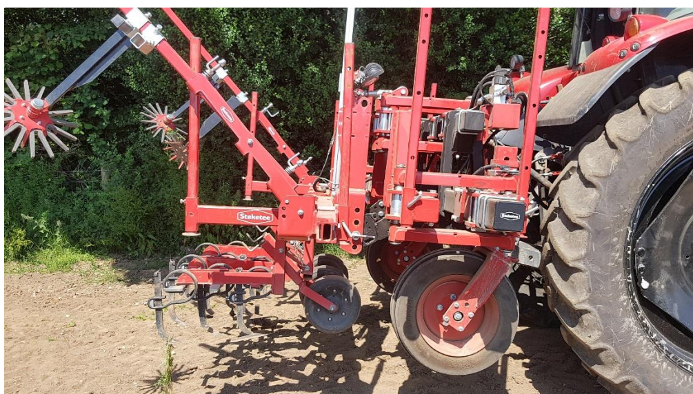
Figure 3. Steketee EC-robotic weeder used at Haverfordwest in 2022. There are cameras attached to the middle section to detect the rows and the tines are on a second section that can be manually adjusted to fit the crop row spacing. Only a one-bed set of times was trialled.
