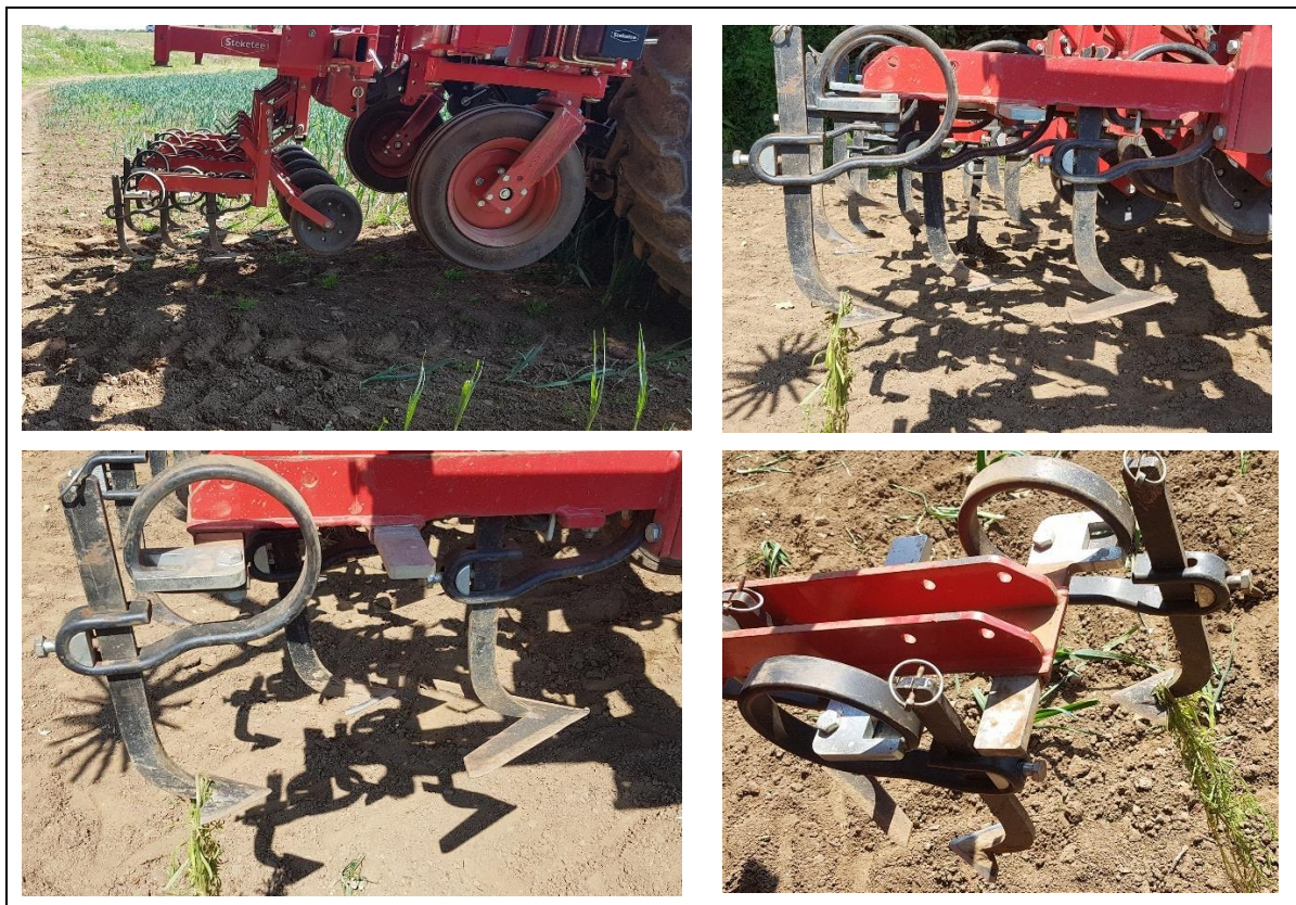
Figure 8. Robotic weeder in leek crop. Various examples of the blades lifting weeds.
