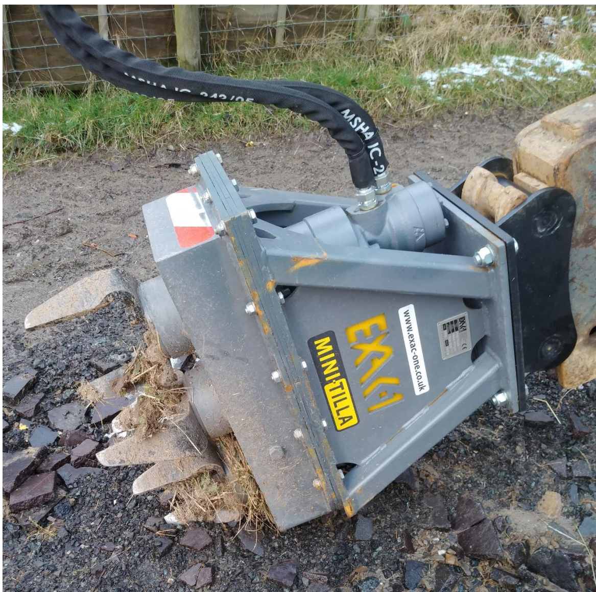
Ffigur 4: Atodiad peiriant palu Minitilla
