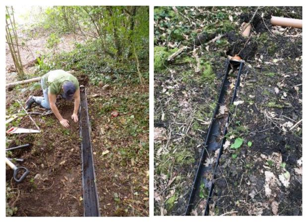
Figure 20 Guttering embedded at the soil surface to capture downslope runoff
