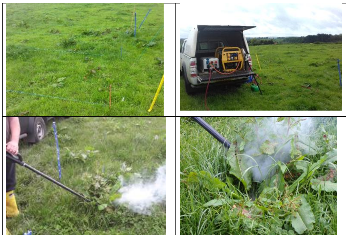
Figure 3 Photo examples of the trials in spring 2019. Top L: field plot markers; Top R: The electrical weeder 'Rootwave Pro' kit in the truck; Bottom L: Lance treating a dock plant; Bottom R: Close up of lance treating dock plants.
