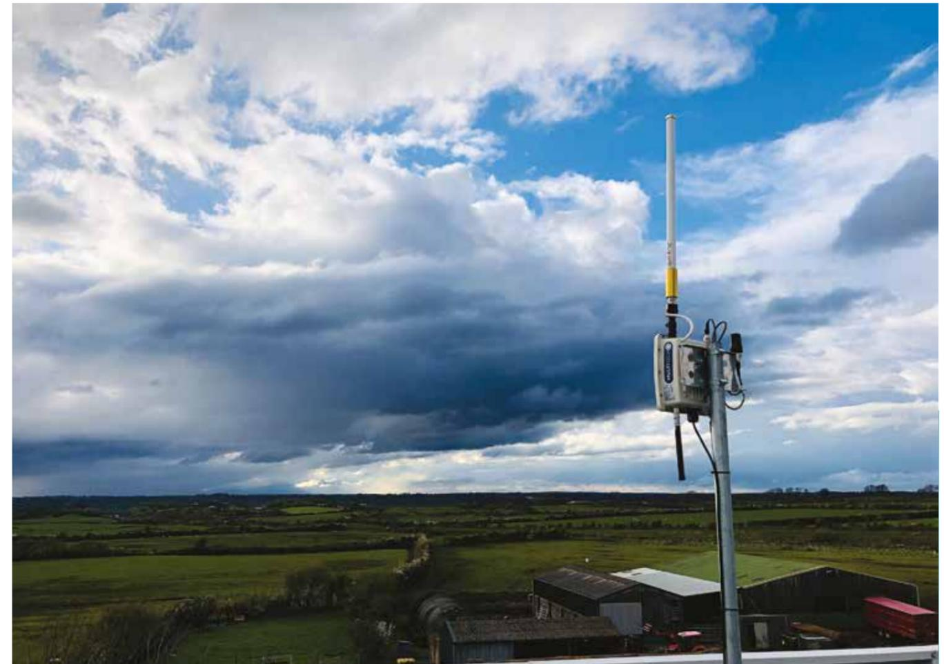
A LoRaWAN gateway (aerial) that can be installed outside, on a roof of a shed for example.
