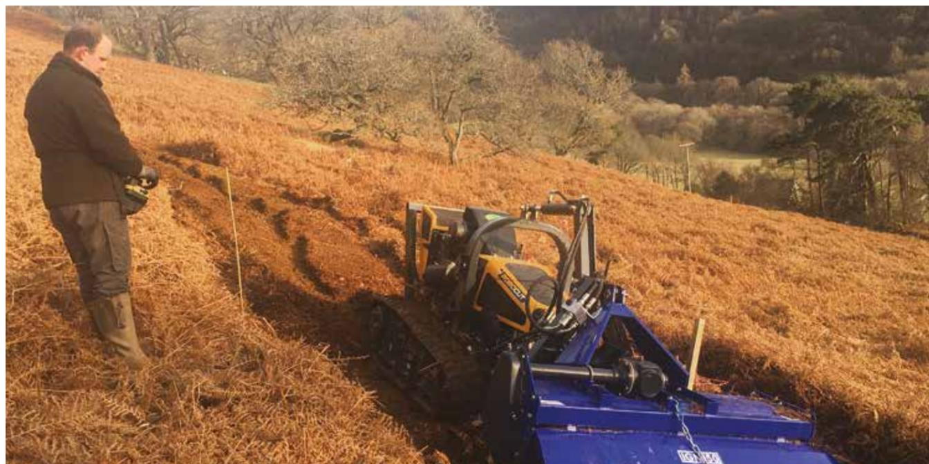
The remote controlled Robocut machine with a cultivator attachment
