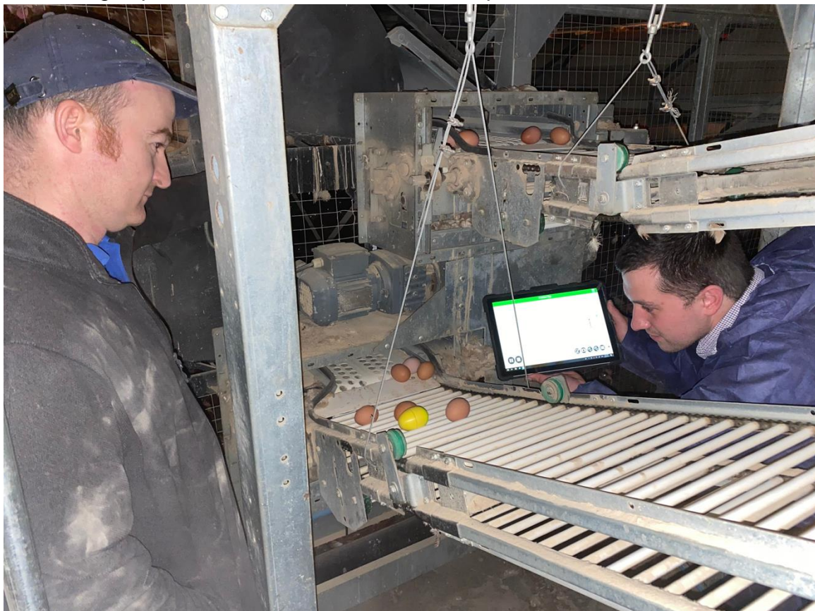
Figure 17. Osian and Gwesyn measuring impact of force at one of the transfer points
