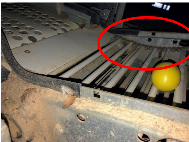
Figure 6. Sag in belt on transfer point 1
