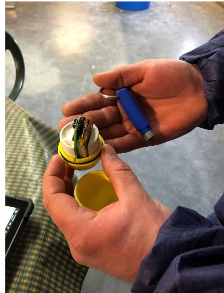
Figure 2. Inside the CracklessEgg™ device are sensors
