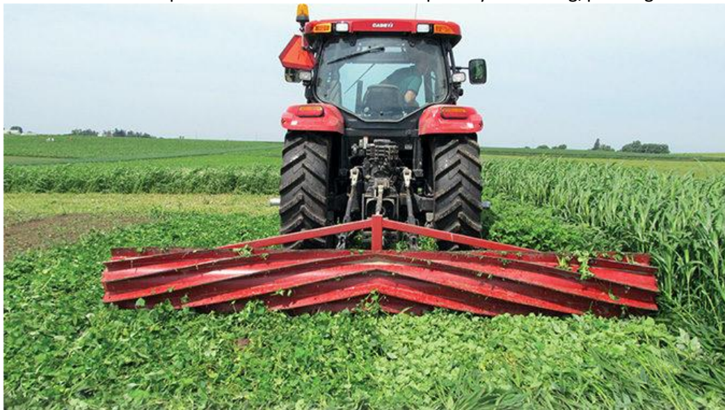
Roller crimper – to knock back a cover crop ready for drilling/planting
