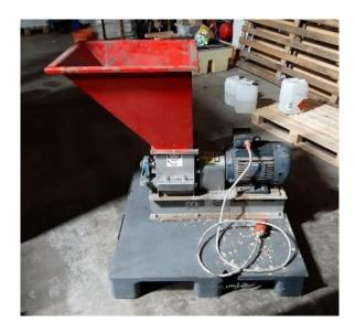
The organic matter needs to be filtered out of the solvent prior to onward processing. The following picture shows a mobile screw press unit that could be used to recover the remaining solvent from the filtered biomass and thus improve recovery yields.
