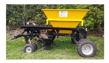
While squill bulbs are significantly larger than daffodil bulbs, the design of this machine is such that it would be readily adapted to planting squill bulbs.
