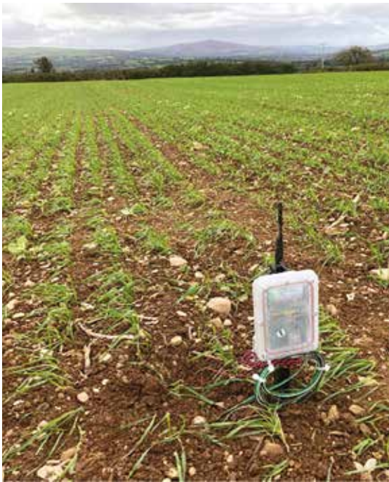
Figure 5: Set of soil nitrate, temperature and moisture sensors with LoRaWAN transmitter
