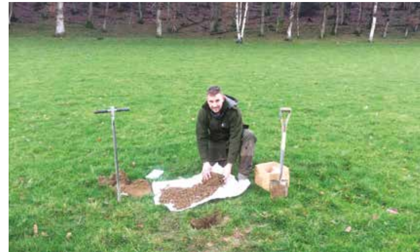
Figure 1. Tom Evans undertaking a visual evaluation of soil structure.
