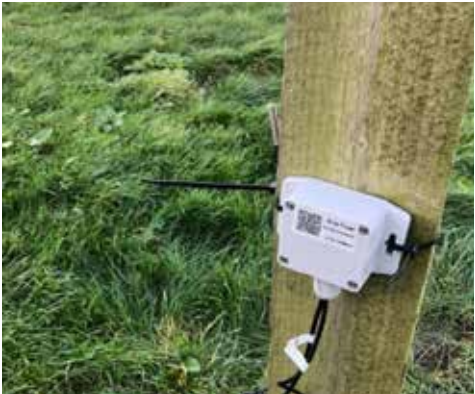
Figure 1. Dual temperature sensor fitted to paddock post. One probe is set 6 inches below ground while a second probe is tied to the fence post.
