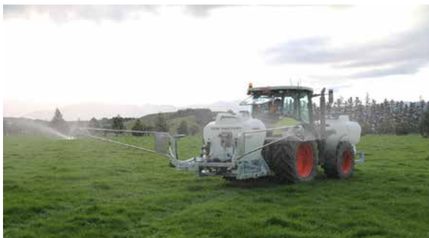
Figure 1. A 'Tow and Fert' sprayer specifically designed to apply liquid fertiliser.
