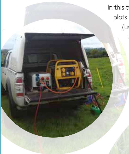
The Rootwave Pro machine uses a petrol generator and hand-held lance with a long (~20m) cable.
