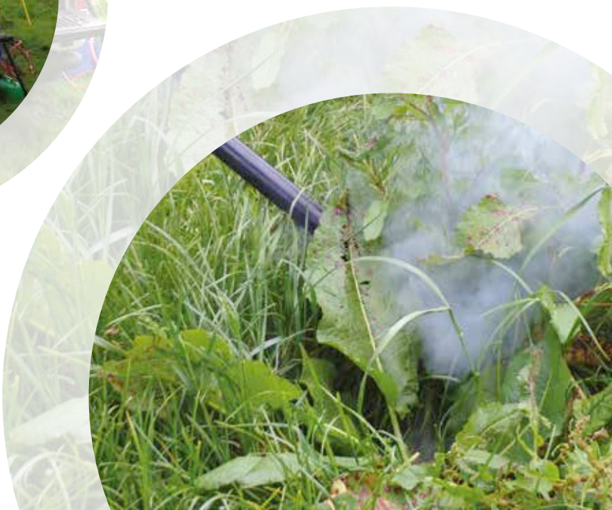
The Rootwave Pro machine uses a petrol generator and hand-held lance with a long (~20m) cable.
