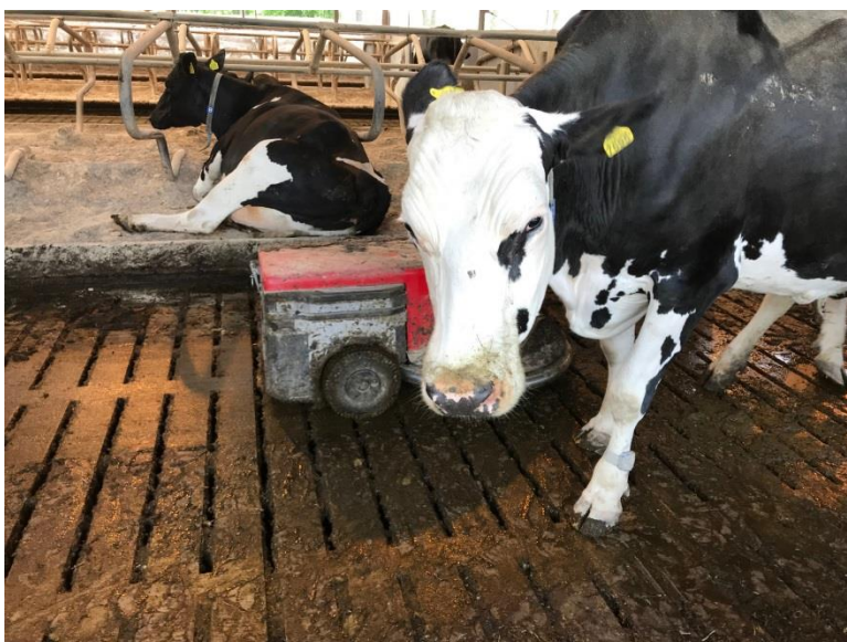
Pre-programmed scraper robot. Works well in winter, but when the slurry partially dries in the summer, it is not as efficient.
