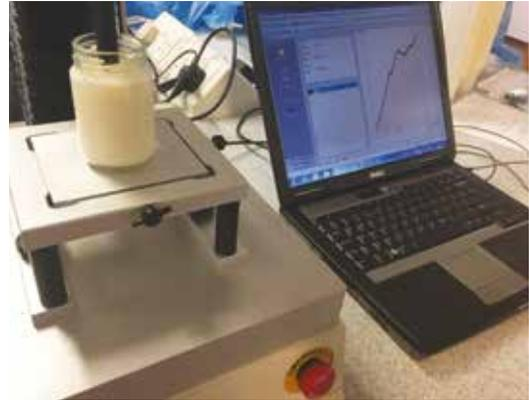
Fig 2. Texture analyser assessing firmness and coagulation
