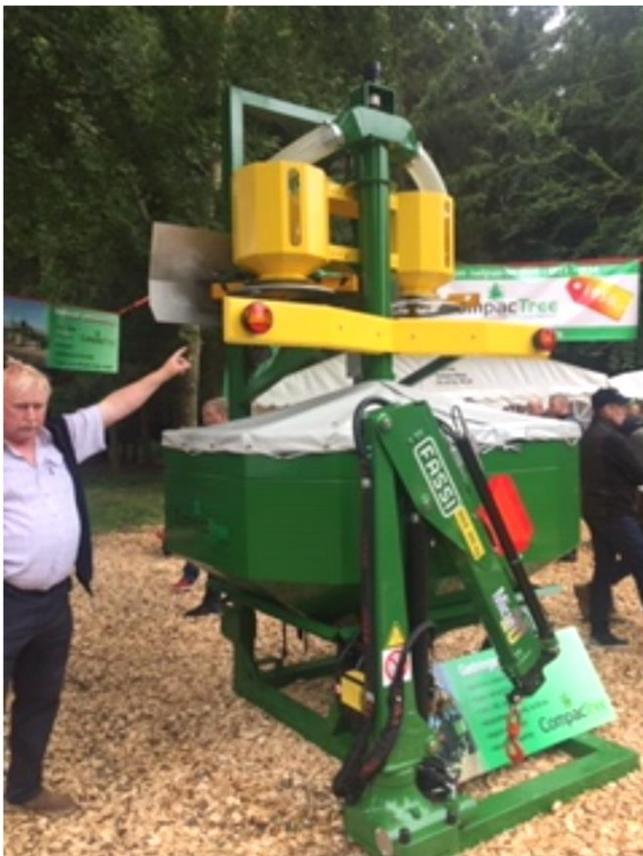
Fertiliser spreader with discs at top to go over trees.
