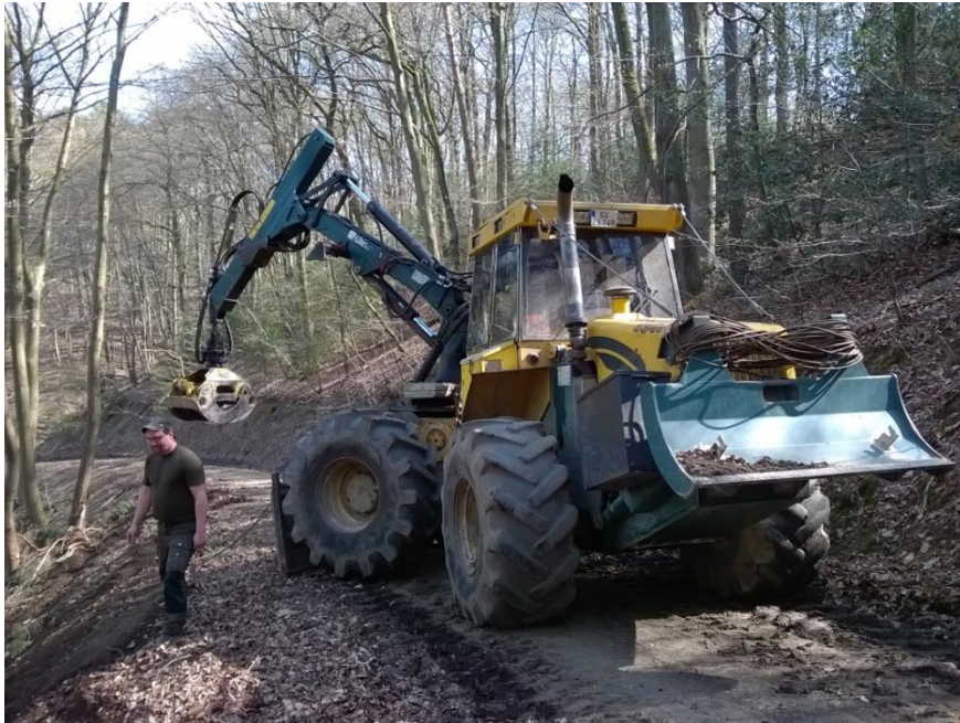
A winch tractor with timber grab. Note that the vehicles stay on the forest road, and band tracks are not required.
