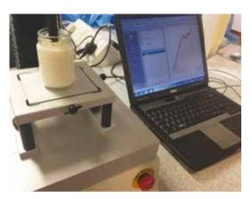
Fig 2. Texture analyser assessing firmness and coagulation
