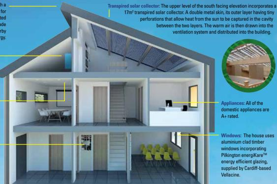
Structure/walls: Use of 194mm Structural insulated panels (SIPS) 150mm is standard. U-value (a measure of heat loss) is just 0.14 for these panels. External wall render minimises risk of thermal bridging and brings overall wall U-value to 0.13.
