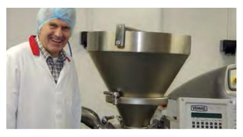
The automatic cake mix depositor – a Reiser Vemag V500 B – was purchased after innovation funding backed by EU funds was secured at the end of 2014. The machine accurately measures and mixes out dough, and has resulted in significant quality and efficiency improvements for the business. Another major benefit of the technology is that it has raised volume without compromising the handmade nature of Tan Y Castell's products - the major selling point of the bakery.
