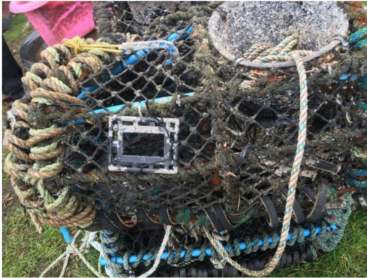
Figure 22: Escape hatches can be easily incorporated into existing fishing pots
