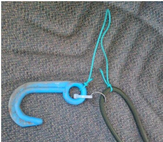
Figure 23: Pot modification example. If the pot is lost, the keyring will begin to rust, and the door of the pot will open thus allowing animals to escape (awarded Sea Change Champion for world animal protection (2015) due to modification).
