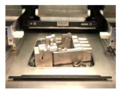
The components produced on the printer are large, dense and capable of withstanding the harsh environment of high pressure die casting. They differ from the traditional 3D printed components that people are more familiar with, which typically have lightweight lattice structures and thin walls.
