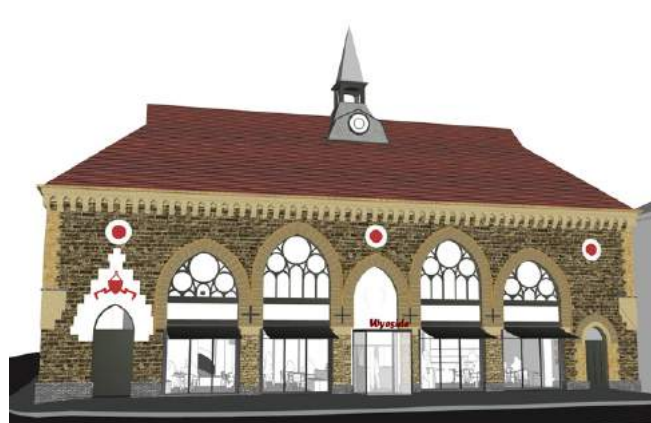
3D study of front street facing elevation with original arches re-opened up and awnings re-established.
