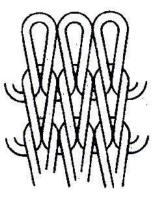
Figure 16 Illustration of knit fabric
