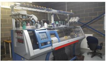
Figure 8 Stoll multi gauge knitting machine, Camira Technical Knit
