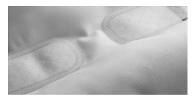
Figure 17 Close up detail of woven airbag [2]
