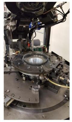
Figure 5 Close up of circular knit needle bed
