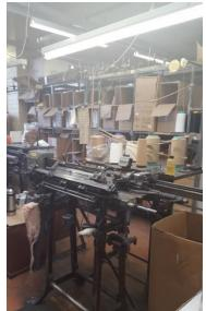
Figure 10 Manual double bed knitting machine utilised at Sallis Healthcare
